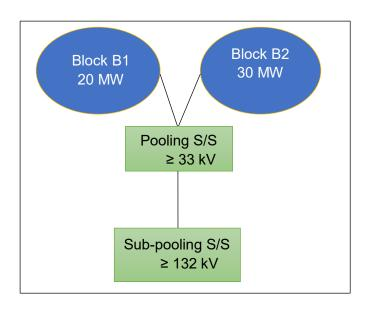
**SOLAR PROJECT COMPONENT CAPACITY: 50 MW**
