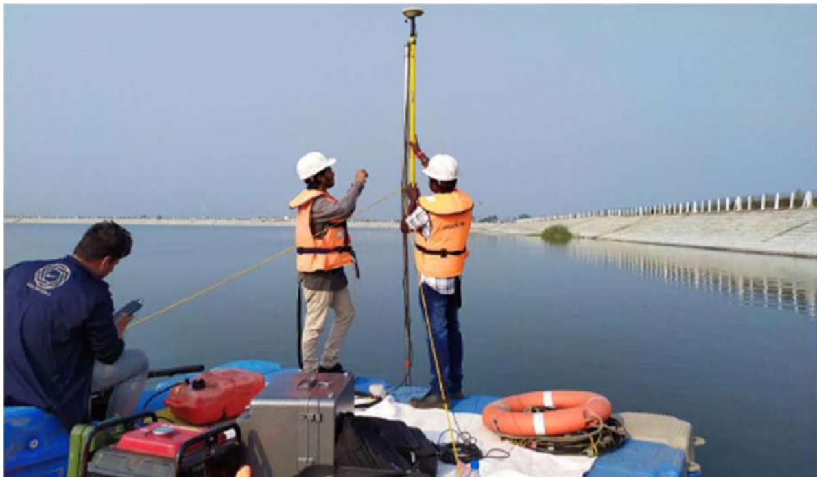
Fig: 8.7: Fixing of GPS at the top of Transducer
