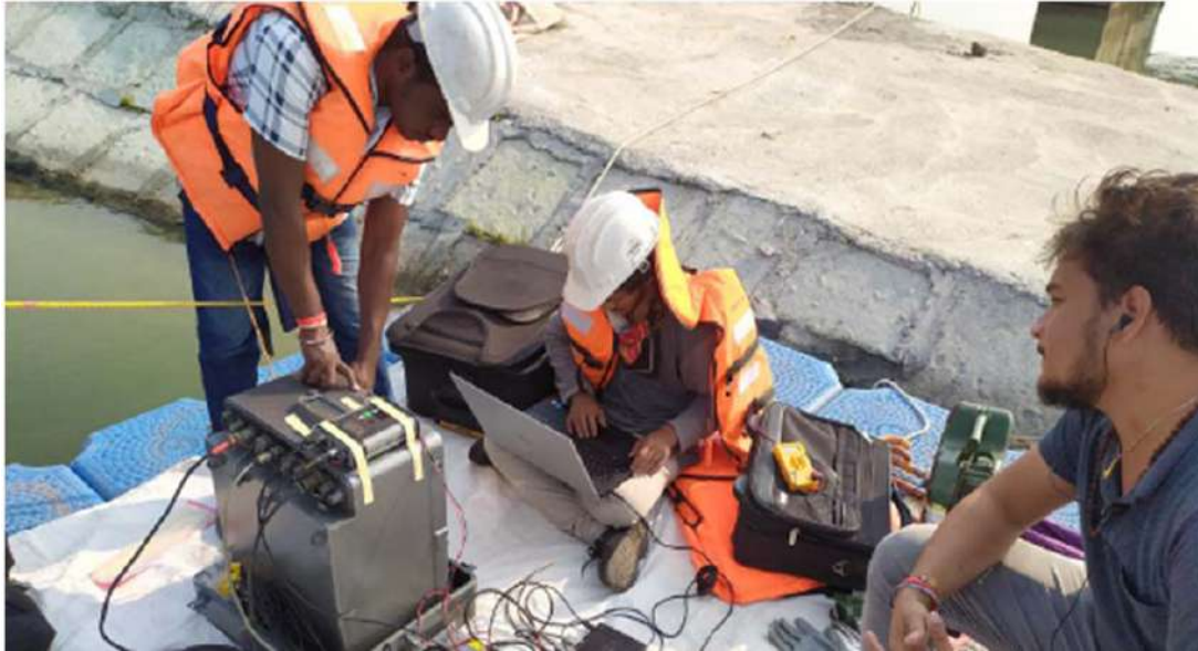
Fig: 8.9: Conducting Echo Sounder Calibration by Bar Check Method
