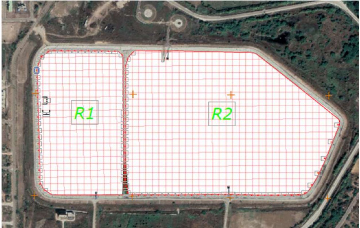
Fig: 3.0 Grid Survey Line
