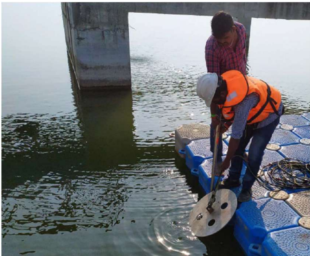
Fig: 8.9: Conducting Echo Sounder Calibration by Bar Check Method
